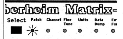
Patches are grouped in ten banks of 100 patches each. The first digit of a patch number is the bank (0 through 9), and the last two digits are the location of the patch within the bank (00 through 99). For instance, patch 427 is bank 4, location 27.
