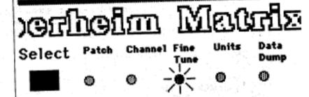
When Fine Tune is selected, the Display reads the current Fine Tune value. This value is stored in memory until it is changed. Change the value by using the + and - keys or the Number keys.
