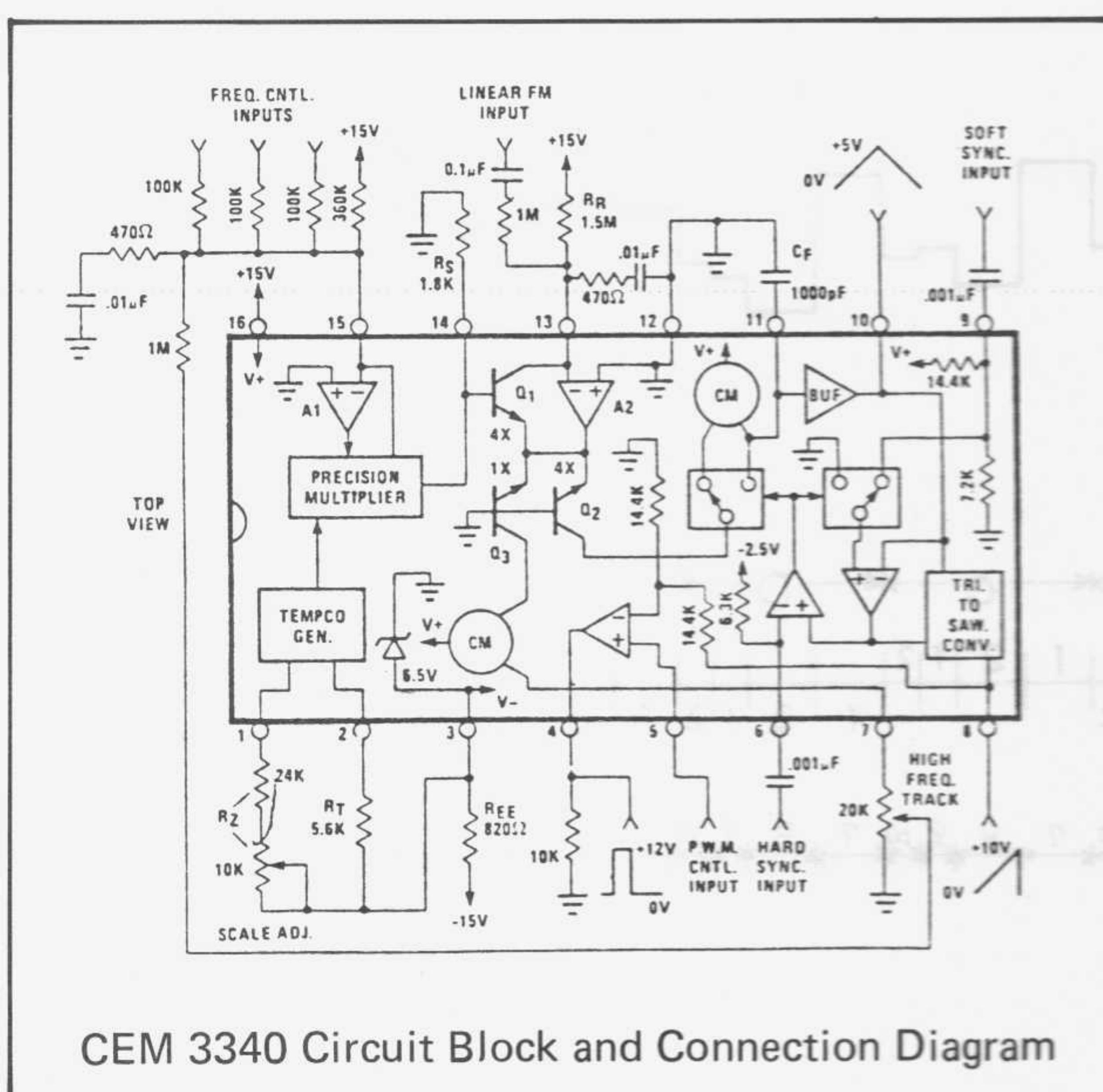
CEM 3340 Circuit Block and Connection Diagram
