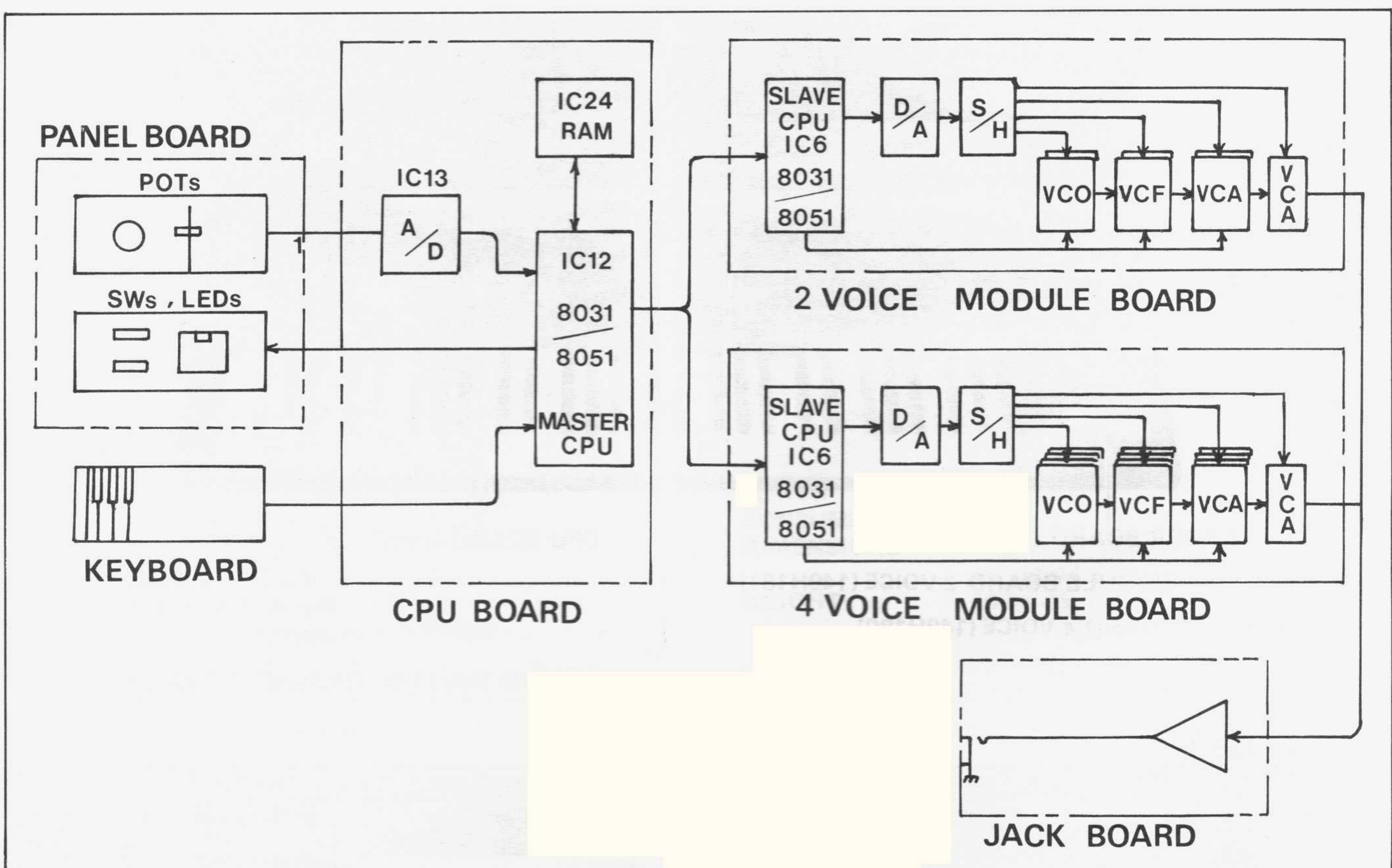
The setting values of the potentiometers on the PANEL BOARDS are converted into digital equivalent by the A/D converter (IC13) on the CPU BOARD, and are read by the MASTER CPU (IC12). The setting values of the switchies on the PANEL BOARDS are directly read by the CPU through the Matrix circuits divided into the two PANEL BOARDS. The CPU (IC12) writes these data into RAM (IC24). The data in the RAM are read by control operation through the panel when required and
