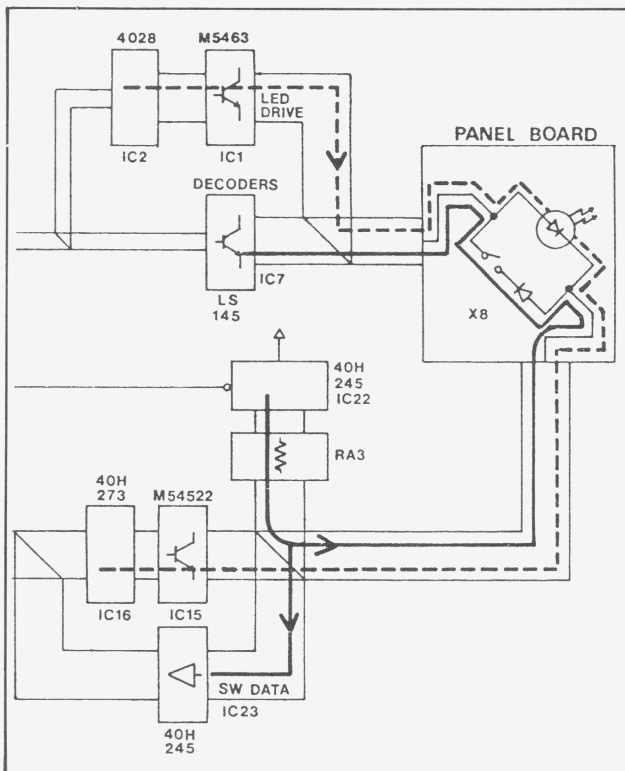
Reading switch states and driving LEDs are alternately repeated through 8 x 8 matrix (divided into the R and L PANEL BOARDS) using a single line.
