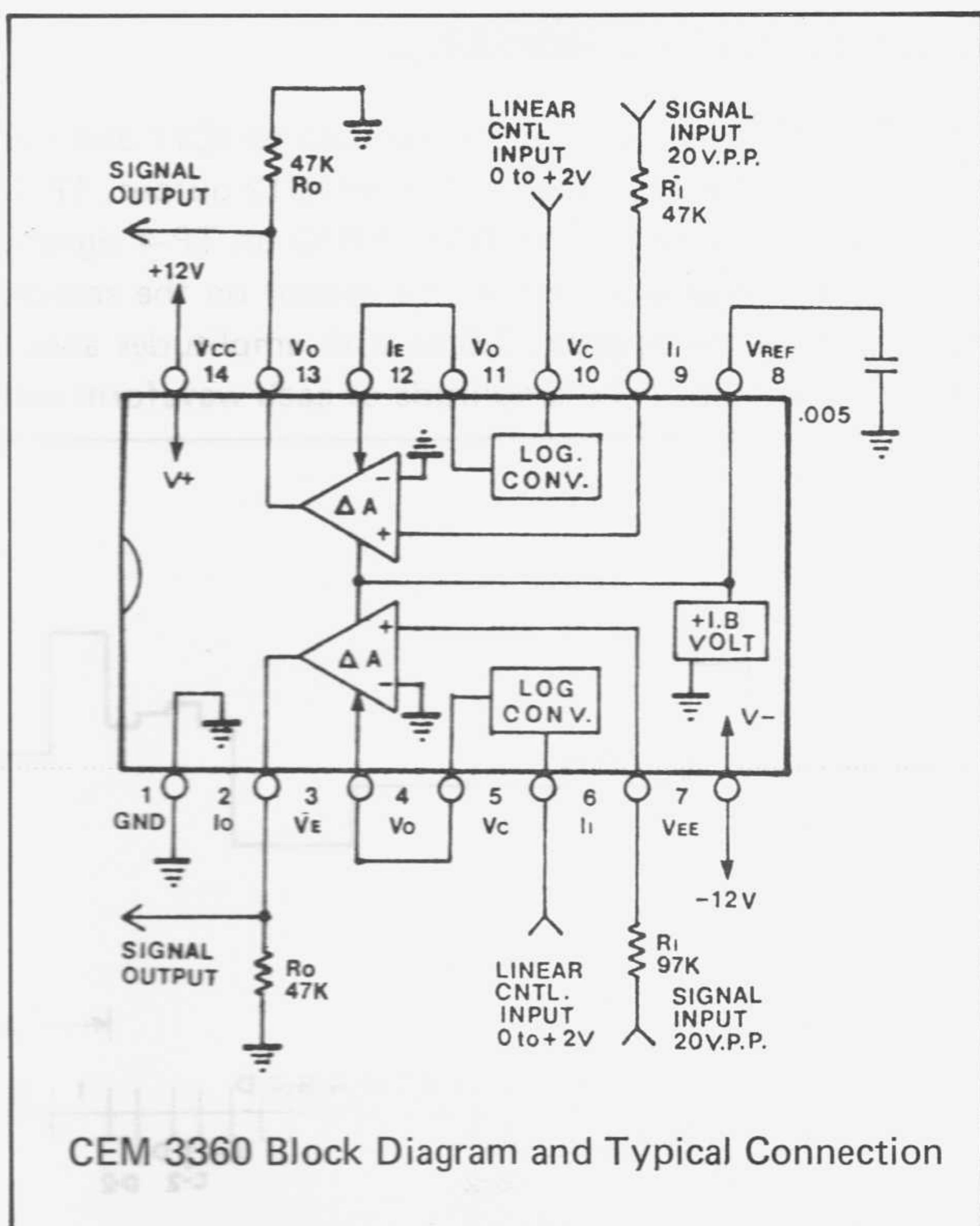
CEM 3360 Block Diagram and Typical Connection
