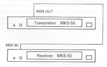
\*Before taking the above procedure, set the MIDI channel of the receiver to the same number as the transmitter's.
