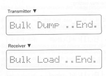
When the data is not received, the receiver shows "Load Error". Check if the connections are correctly and securely made, then repeat the transfering procedure.
