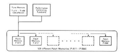
As shown in the picture below, Patches are divided into two Groups A and B, and each Group containes 8 Banks and 8 Numbers.
