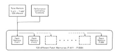
As shown in the picture below, Patches are divided into two Groups A and B, and each Group containes 8 Banks and 8 Numbers.
