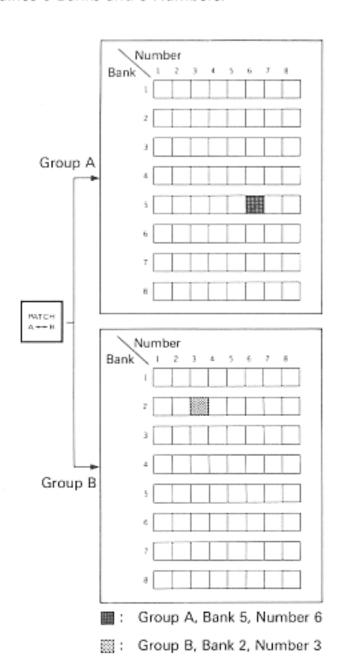
The Display shows the Patch in the combination of an alphabet and a number such as A56, B23 etc.
