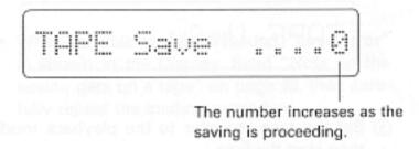
6 If your tape recorder features recording level control, set the level so that the meter will read 0 VU while "0" is shown in the Display.
