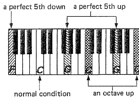
1. If you press a key lower than the lowest C, it will be transposed down by the distance in pitch between the pressed key and the C.
