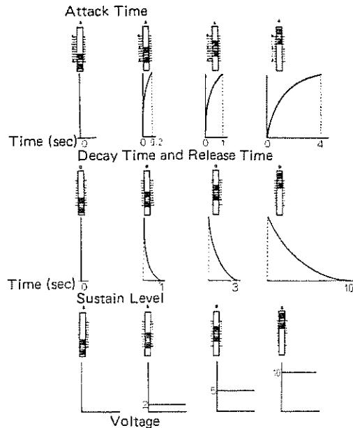
\* In the figure shown above, the positions of the knobs are not meant to be exactly correct, so the knob position does not necessarily correspond with the time and the voltage.
