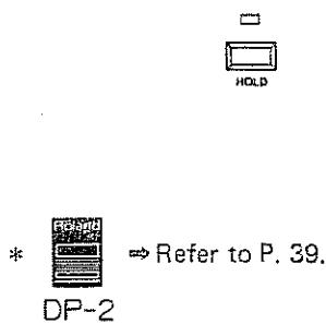
You can hold the sound even after the key is released, by pressing the HOLD button (the indicator lights up). The level of the sound is determined by the Sustain level of the Envelope Generator. Therefore, Hold function is not obtained if the Sustain level is zero (Decay sound). The Pedal Switch (DP-2, sold separately) functions like a damper pedal of a piano.
