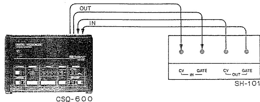
\* As soon as the external unit is connected to the CV IN and GATE IN, internal connection of CV and GATE will be automatically cut.
