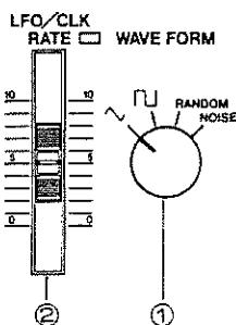
The LFO also provides the output waveform of  $\sim$  which controls the VCO and VCF by using the BENDER in the Controller Section.
